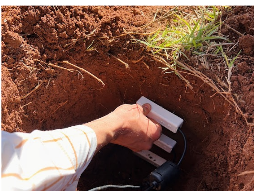
Installing soil moisture & temp sensors
